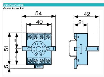
Screw terminal or connector socket - 8-pin base : ref. 25 622 303 - for mounting on DIN rail 35 mm EN 50022
