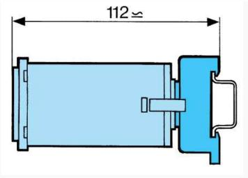
Screw terminal or connector socket - 8-pin base : ref. 25 622 303 - for mounting on DIN rail 35 mm EN 50022
