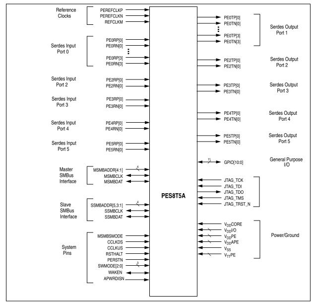
Figure 4 PES8T5A Logic Diagram
