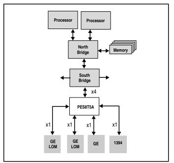
Figure 2 I/O Expansion Application
