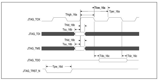
Figure 6 JTAG AC Timing Waveform
