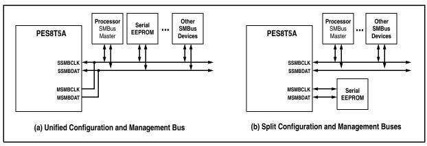
Figure 3 SMBus Interface Configuration Examples
