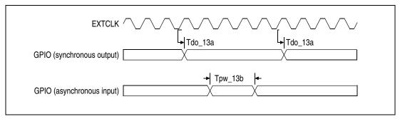
Figure 5 GPIO AC Timing Waveform
