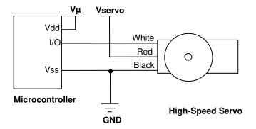
$V\mu$  = microcontroller voltage supply
