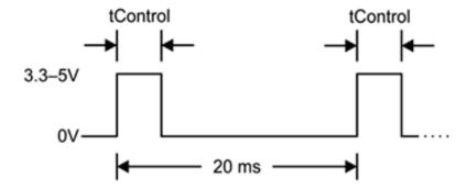
The duration (pulse width) of tControl determines servo rotation speed and direction as shown in the table below. The top speed will vary with supply voltage and load.
