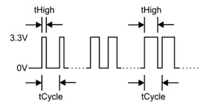
Duty cycle corresponds to the rotational position of the servo, in the units per full circle desired for your application.
