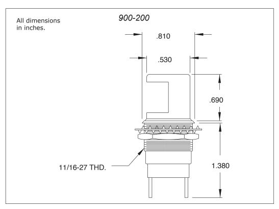
Chicago Miniature Lamp Instrument Lites are specifically designed to provide localized light for illuminating panels, meters, switches and legends. The Chicago Miniature Lamp Instrument Lite features a highly reflective surface on the inside of the hood to assure peak light output and is easily relamped from the front of the panel. The lamp is not included with this indicator light; please order the required lamp separately.
