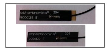
Ethertronics' Prestta series of Isolated Magnetic Dipole $^{\mathbb{M}}$  (IMD) trace antennas address the challenges facing today's product designers. IMD's high performance and isolation characteristics offer better connectivity and minimal interference.
