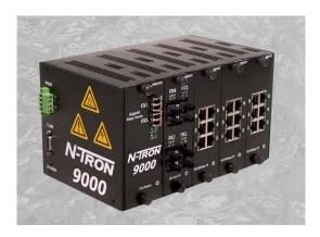
**Port Mirroring** - This function allows the traffic on one port to be duplicated and sent to a designated mirror port. Port mirroring can be used to monitor Ethernet traffic on the designated source port using the assigned mirror port.
