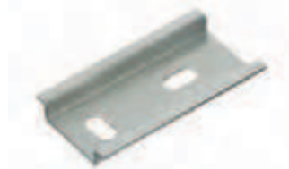
TS 35/7.5 mm according to EN 50022 (s = 1.0 mm)
