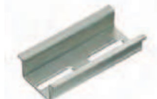
TS 35/15 mm according to EN 50022 (s = 1.5 mm)
