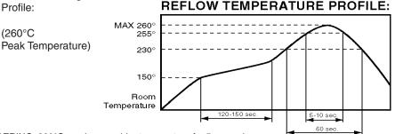
WAVE SOLDERING: 260°C maximum solder temperature for 5 seconds max. \*\* Note: 100% matte tin terminal plating does not meet MIL-S-83504 for lead content.
