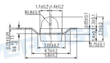
Note: The tolerances unless mentioned are ±0.1, unit=mm.
