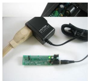
Take the board out of the vise and plug in a power source such as a 9V DC positive-tip wall adapter or a 9V battery with a 2.1mm barrel jack. You should see the green LED light up.
