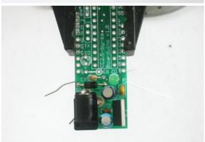
Solder in the resistor and LED and clip the leads.
