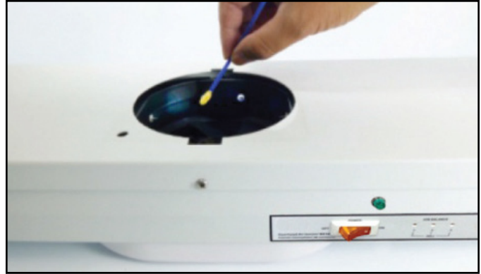
Figure 8. Wipe the emitter tips, brushes and fan blades with a cotton swab or brush. After cleaning, re-install the front grill and the screws.
