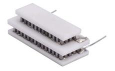
This product line is available in numerous heat pumping capacities, geometric shapes and temperature differentials. Assembled with Bismuth Telluride semiconductor material and thermally conductive Aluminum Oxide ceramics, the MS Series is designed for higher current and lower heat-pumping applications.
