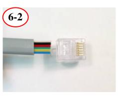
Insert cable into plug observing correct wire order
