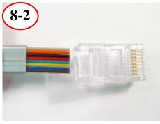
Insert cable into plug observing correct wire order
