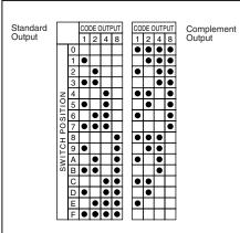
Dot indicates terminal to common connection. All switches are continuous rotation.
