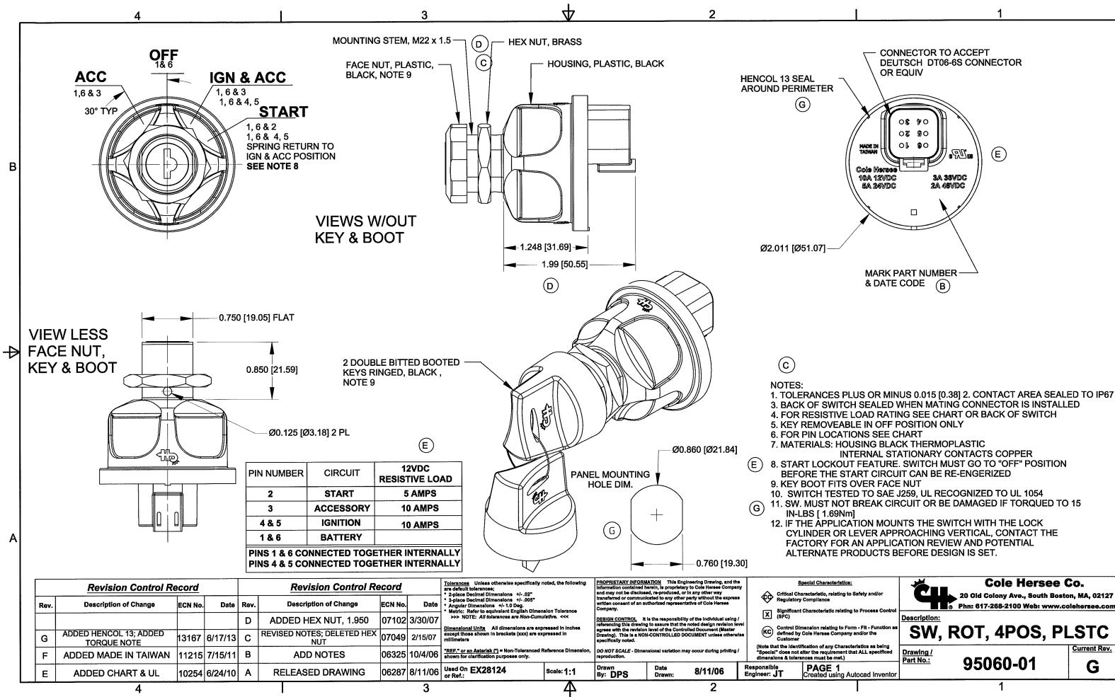
INTERNAL STATIONARY CONTACTS COPPER Cole Hersee Co. 20 Old Colony Ave., South Boston, MA, 02127 Phn: 617-268-2100 Web: www.colehersee.com SW, ROT, 4POS, PLSTC Current Rev.
