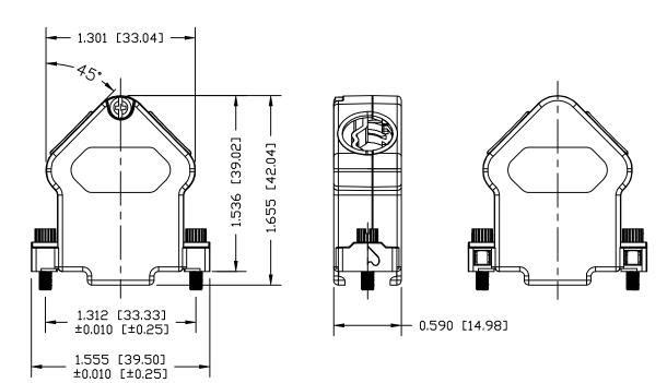
MATERIAL: **DIE-CAST ZINC ALLOY NICKEL OVER COPPER** PLATING: STEEL, ZINC PLATED JACKSCREWS: **HOUSING SCREWS:** STEEL, ZINC PLATED STEEL, ZINC PLATED **STRAIN RELIEF SCREWS:** STEEL, ZINC PLATED **COVER PLATE:** STRAIN RELIEF CLAMP: STEEL, ZINC PLATED
