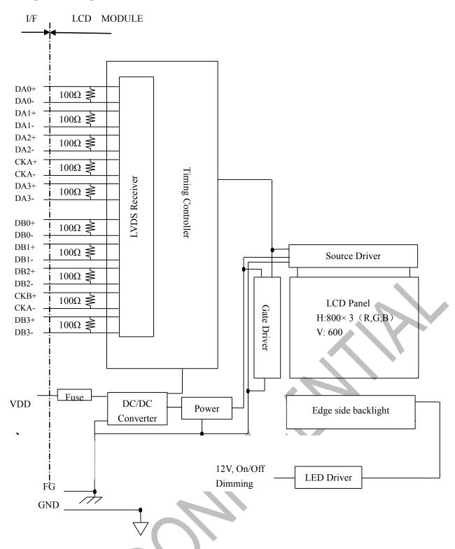
Note: System ground (GND), FG (Frame ground) in the product should be connected together in customer equipment.
