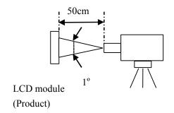
Luminance Meter (TOPCON BM-5A) Spectroradiometer (TOPCON SR-3)
