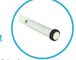
970 Series non-relampable snap mount indicator lights feature molded plastic flex arms which ensure easy front panel installation into a 5/16" diameter hole.
