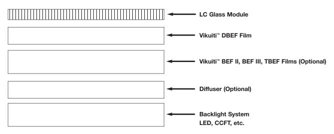
The film must be mounted with its transmission axis parallel to the transmission axis of the rear polarizer.
