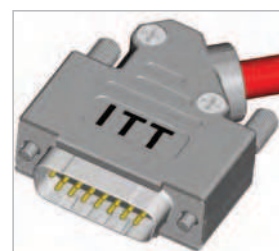
Assemble the other half (screwing force: 100-120 Ncm)
