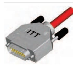
Assemble the other half (screwing force: 100-120 Ncm)
