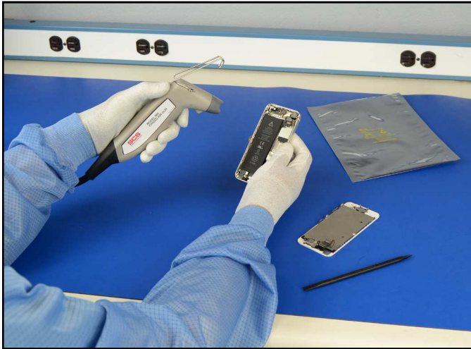
Figure 5. Using the Ionized Air Gun
