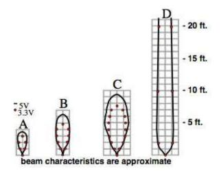
The different LV models have different beam width patterns, check this image for a comparison of all the LV model beam patterns. For higher sensitivity, check out the HR-LV models – they have up to 1mm sensitivity and 5 meter range!
