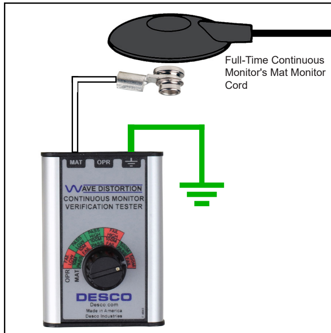
Figure 11. Connecting the Wave Distortion Monitor Verification Tester to the Full-Time Continuous Monitor's mat monitor cord
