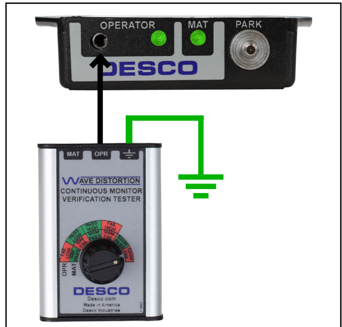
Figure 6. Connecting the Wave Distortion Monitor Verification Tester to the Mini Monitor's operator jack
