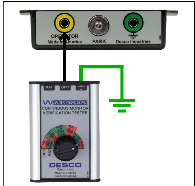
Figure 8. Connecting the Wave Distortion Monitor Verification Tester to the satellite remote's operator jack
