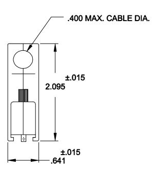
**METALIZED PLASTIC: MATERIAL: ABS HIGH TEMPERATURE PLASTIC 94HB METALIZED PLATING:**
