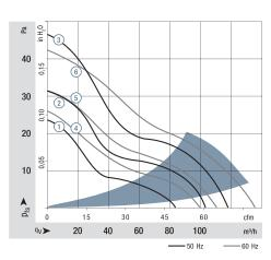
Air performance measured according to: ISO 5801. Installation category A, without contact protection. Noise: Total sound power level  $L_WA$  ISO 103002 measured on a hemisphere with a radius of 2 m. Sound pressure level LpA measured at 1 m distance from fan axis. The values given are applicable only under the specified
