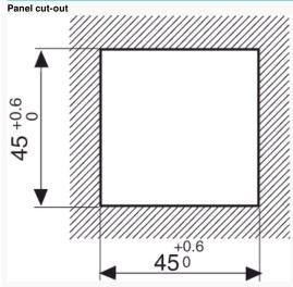
Dimensions (mm) 26546842 - Adaptor for 72 x 72 mm cut-out
