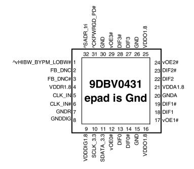
**32-pin VFQFPN, 5x5 mm, 0.5mm pitch** ^ prefix indicates internal 120KOhm pull up resistor
