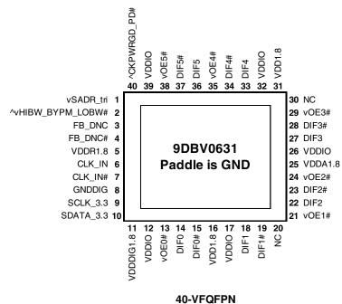
^ prefix indicates internal Pull-Up Resistor
