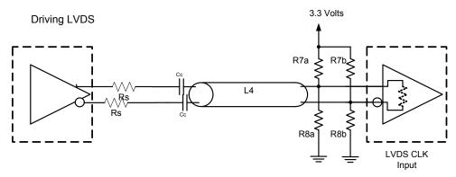
Driving LVDS inputs with the 9FGV0231
