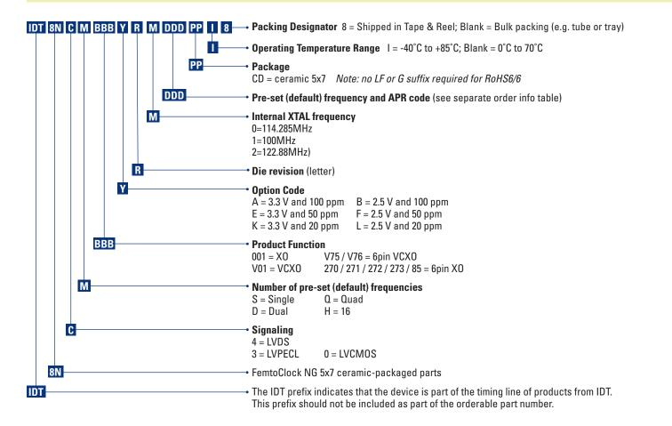
Example: IDT 8N3Q001LG-0001CDI8 is a LVPECL FemtoClockNG programmable oscillator, quad output frequency (125, 100, 122.88, 156.25 MHz), 2.5 V, 20 ppm, G-revision, 114.285 MHz XTAL in a RoHS 6/6 ceramic 5x7 package with tape and reel.
