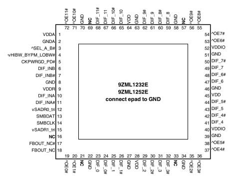
^ prefix indicates internal 120Kohm Pull Up v prefix indicates internal 120Kohm Pull down 10mm x 10mm 72-VFQFPN 0.5mm pin pitch
