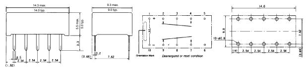
AL-D type (Double winding latching type)
