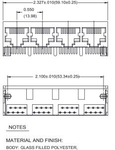
BODY: GLASS FILLED POLYESTER, UL94V-0 RATED CONTACTS: PHOSPHOR BRONZE(0.45mm DIA.) SELECTIVE GOLD ON CONTACTS AS PER PART NO. TABLE, TIN ON TERMINATION, ALL OVERNICKEL UNDERPLATE. SHIELD: 0.25mm THICK COPPER ALLOY PLATED WITH NICKEL
