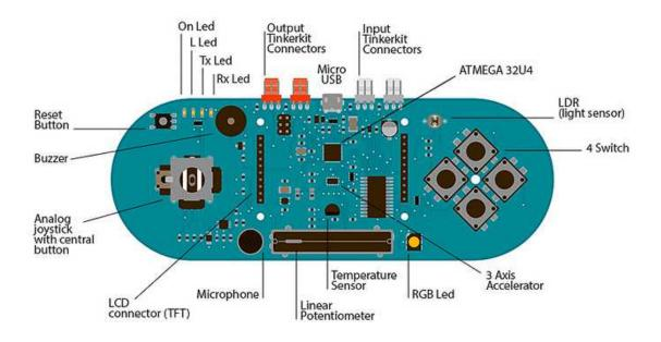
The design of the Esplora board recalls traditional gamepad design with an analog joystick on the left and four pushbuttons on the right.
