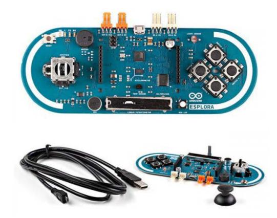
The Arduino Esplora is an Arduino Leonardo based board with integrated sensors and actuators
