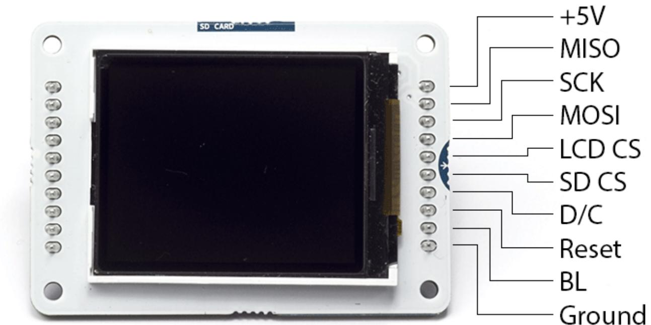
The screen is 1.77" diagonal, with 160 x 128 pixel resolution. The TFT library interfaces with the screen's controller through SPI when using the TFT library. Refer to the screen's data sheet for complete details.
