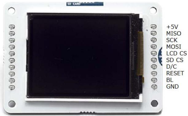
You can either connect the screen with hardware SPI pins, or define your own set of pins. Using the hardware SPI is faster when drawing to the screen.
