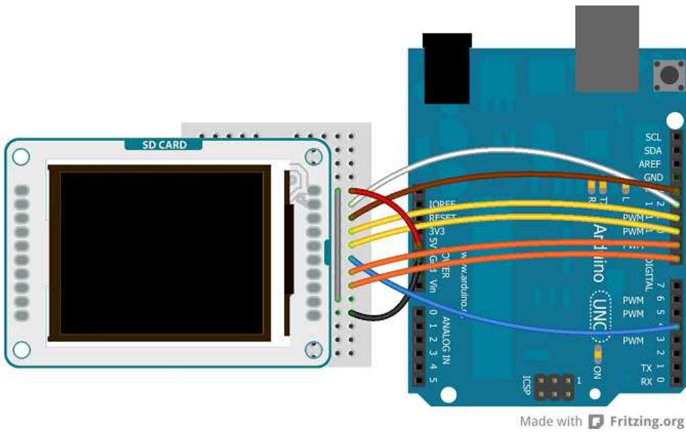
Connecting the pins in the proper way, you can see the lcd screen working with your Uno (or Duemilanove) just uploading the simple "*TFTBitmapLogo*" sketch.
