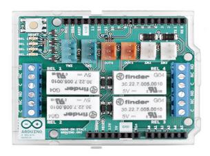
The Arduino 4 Relays Shield allows your Arduino driving high power loads that cannot be controlled directly by Arduino's digital pins. The Shield features four relays, each relay with 2 pole changeover contacts (NO and NC). Four LEDs indicate the on/off state of each relay.
