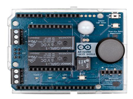
Arduino Lucky Shield is an easy way to use your Arduino boards, that grants you access to barometric pressure, relative altitude, luminosity, temperature, motion and presence. You can also turn it into a simple controller and OLED (organic light-emitting diode) display system. It is the perfect shield for IoT.
