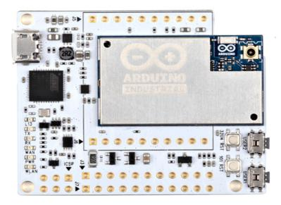
The Arduino Industrial 101 is a break-out board for the Arduino 101 LGA module. Just like the YUN, it integrates an ATmega32U4 and an Atheros AR9331 with WiFi and Linino OS.
