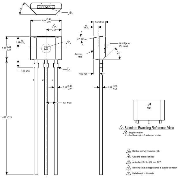
Figure 5: Package UA, 3-Pin SIP
