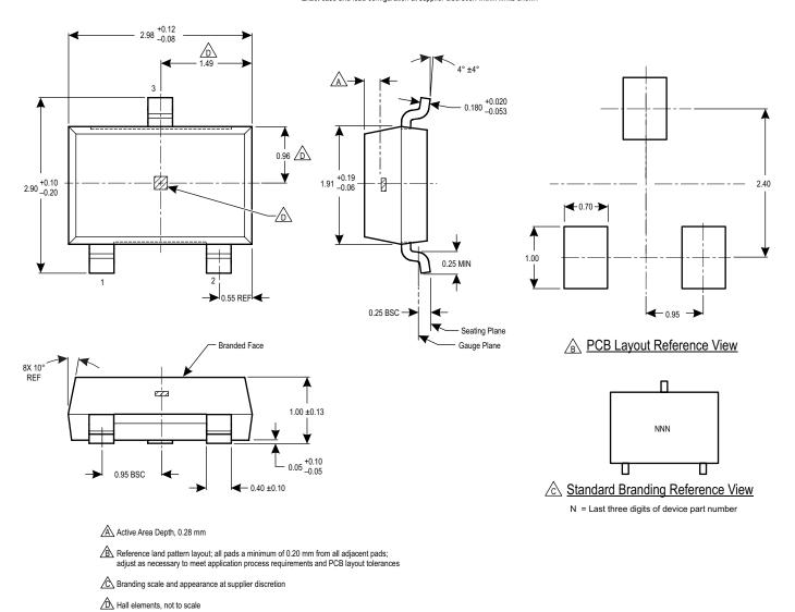
Figure 4: Package LH, 3-Pin SOT23W
