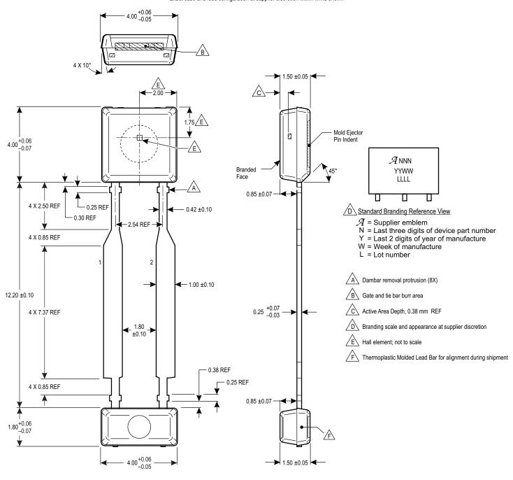
Figure 6: Package UB, 2-Pin SIP
