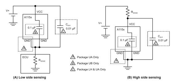
**Figure 2: Typical Application Circuits**
