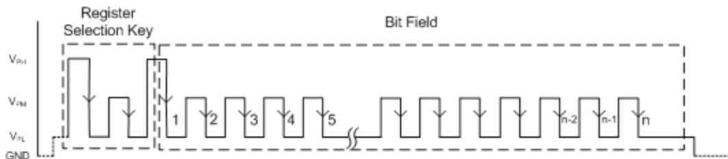
Figure 11. Example of Try mode pulse sequence, Register Key = B OP selection down counting
