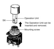
Tighten the hexagonal nut while securing the Switch by holding it with your fingers. Tighten the hexagonal nut with a torque of 0.49 to 0.98 N·m.
