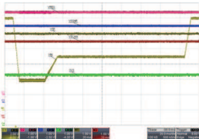
Figure 1: Buck-Boost Performance with Relatively Fast V_{IN} Transition Times for a Representative Start/Stop Waveform
