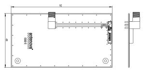
The testboard is designed for evaluation purposes for Mica 2.4 GHz SMD antenna. The board has the same size as a typical PCMCIA card and is fitted with an SMA connector.
