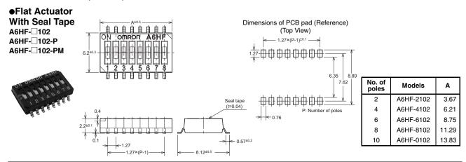
**Note:** Unless otherwise specified, a tolerance of  $\pm 0.4$  mm applies to all dimensions.
