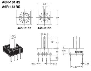
■ Top-actuated Extended-actuator Models with 3×3 Terminal Arrangement
