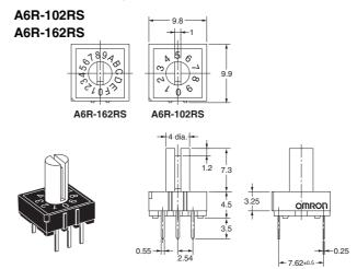
■ Side-actuated Extended-actuator Models with 4×1 Terminal Arrangement
