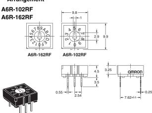
Side-actuated Flat Models with 4×1 Terminal Arrangement
