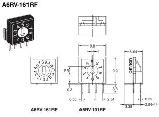
● Top-actuated Extended-actuator Models with 4×1 Terminal Arrangement
