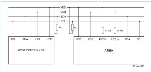
Fig 2. System overview supporting Power-on Reset
