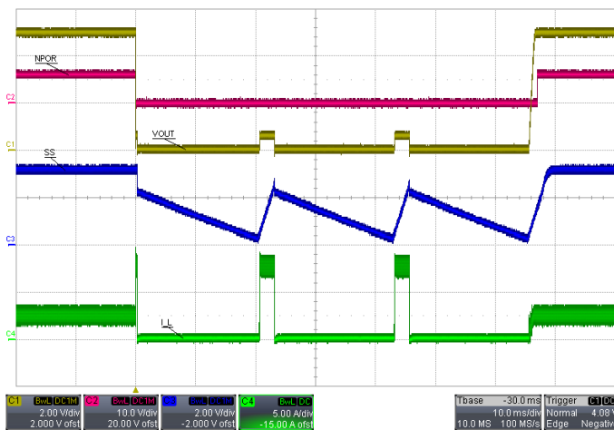
Figure 12: Hiccup Mode Protection and Recovery CH1 = V_{OUT} , CH2 = NPOR, CH3 = SS, CH4 = IL
