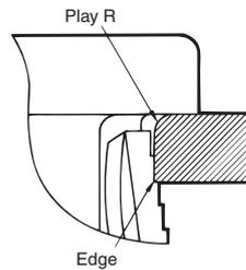
When processing the panel, be sure that the Play R is on the switch operation side.
