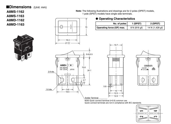
Note: Unless otherwise specified, a tolerance of ±0.3 mm applies to all dimensions.
