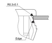
Process the above-mentioned R on the mounting hole side of panel, or be sure that the Play R is on the operation side of panel when using. Be sure that the Edge is on the reverse side of panel when processing.
